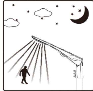
When motion is detected within a 27-33ft range, the ILLS Series will detect that motion and power up to 100%
